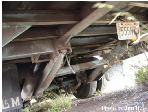
Undercarriage of trailer used to transport backhoe was cleaned and free of soil and dirt.
