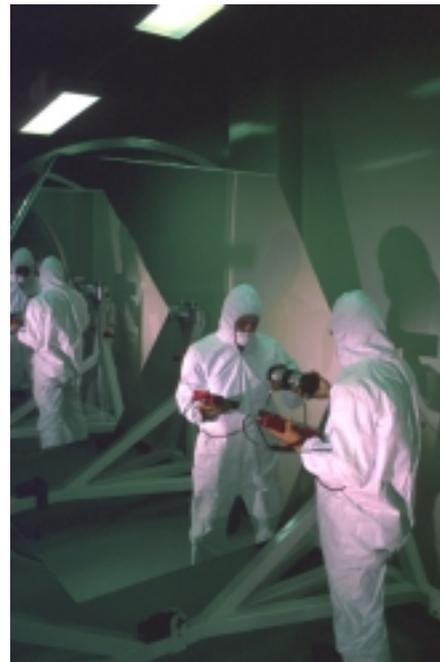
Figure VI-1. Technician testing a mirror segment after washing and recoating. *Photo courtesy of the W. M. Keck Observatory.*
